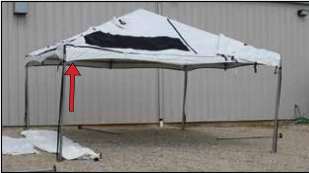
12. Put the other four legs with base plates on the bottom of all of the side tee fittings and pin with pin and bail.
