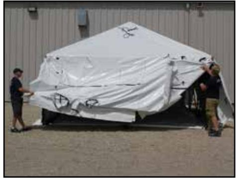
24. Close all corners by connecting all of the side release buckles and tightening.
