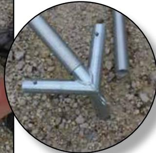
5. Locate and slide all four of the side tee fittings (F02STHT) into the hip rafter poles (Green/HT2GST80). Lining up the holes until the push pins engage.
